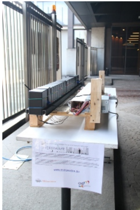
Figure 3.4: Setup of sensor boxes for stationary data collection.
