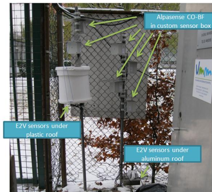
Figure 2.4: 6 Alphasense CO-BF sensors and 2 E2V CO and NO_2 sensors installed on VMM station Plantin En Moretuslei, Antwerp
