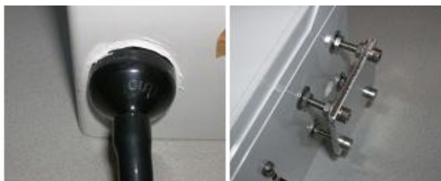
Figure 3.3: Gas inlet tube placed in front of fan (left) and gas outlet protection (right)
