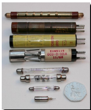
Figure 1.3: Typical Geiger tubes
