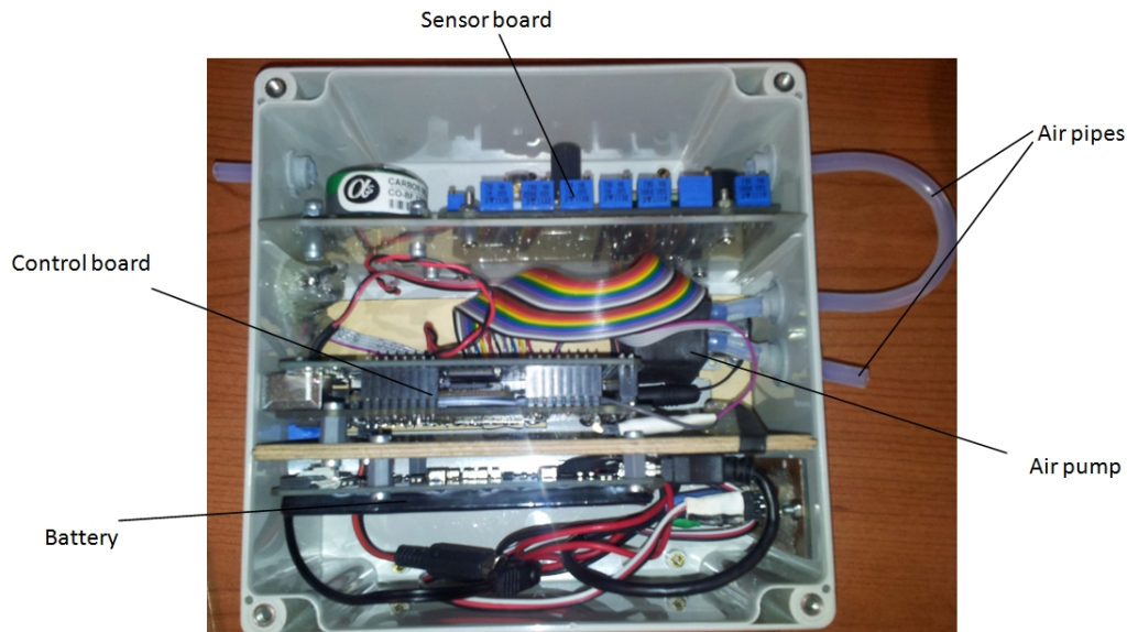
Figure 3.4: Version 1 of the SensorBox packed in a plastic box with holes and pipes for the air flow regulation
