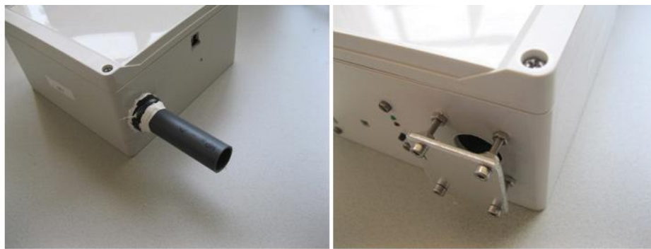
Figure 6.1: Sensor box equipped with wide tube on gas inlet (left) and increased size gas outlet (right)
