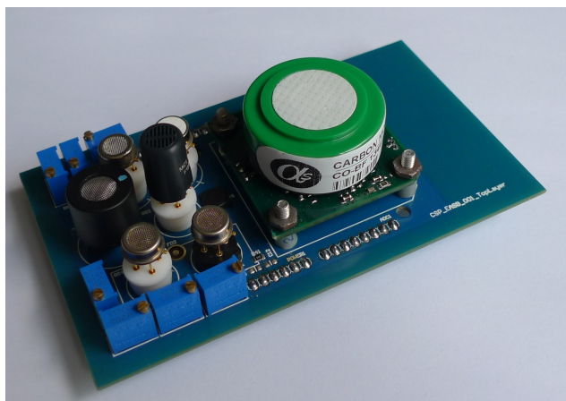
Figure 2.16: The low cost air quality sensors mounted on the sensor shield contained in the SensorBox
