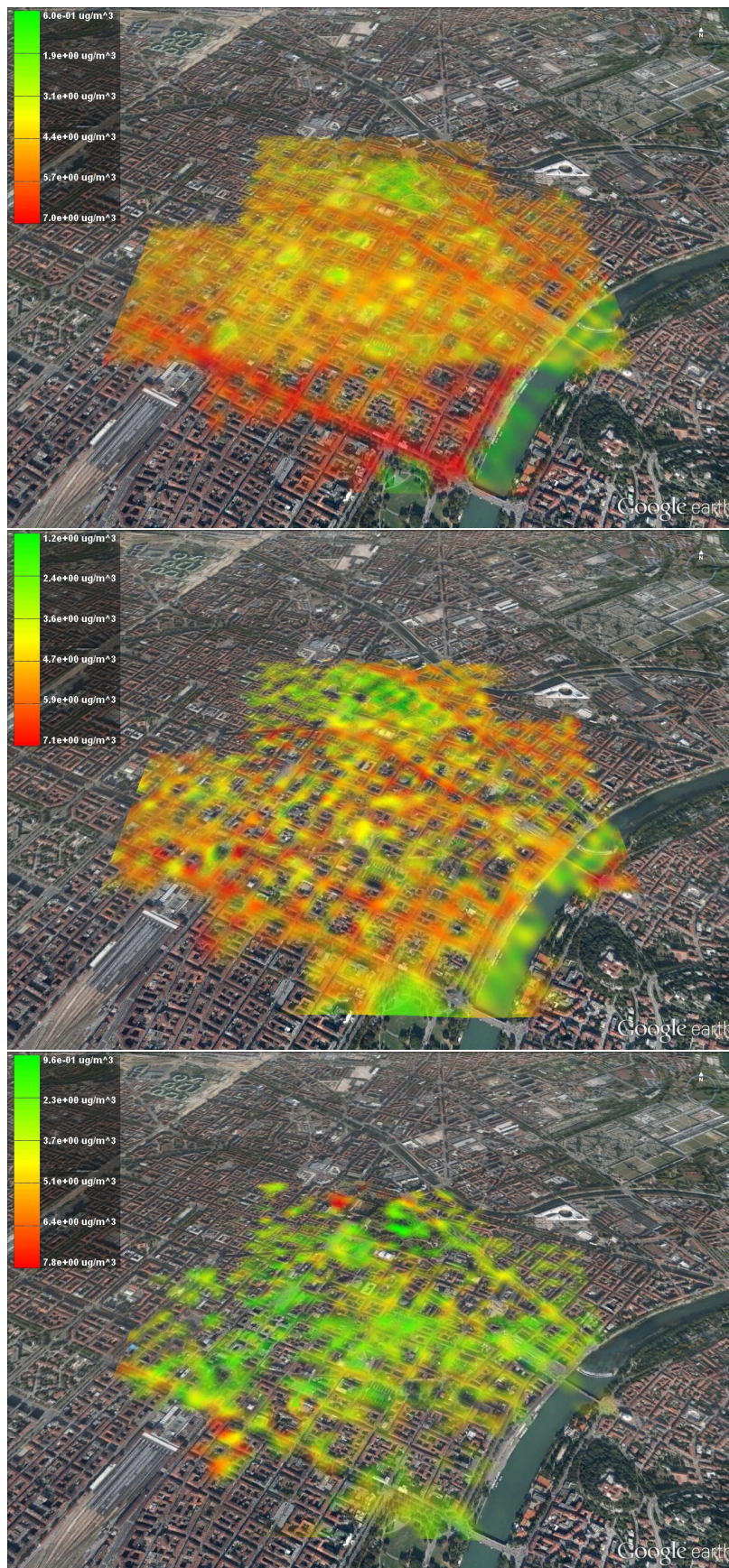
Figure 5.16: From the top, for phase 1, 2 and 3: the heat map of AP values for Turin. Values in the key are, as usual, \mu\text{g}/\text{m}^3 of Black Carbon. The opacity is an related to the number of AirPins in that point.
