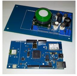
Data gathered from sensors are read by a microcontroller board and stored on SD card. These measurements are saved together with the position given by a GPS module. A Bluetooth module allows the connection with a smartphone to transfer all the data collected for real-time visualization through the smartphone and/or forward to the main server.
