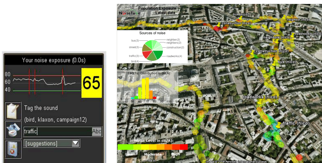
(a) The user interface of the mobile application allowing to measure, tag and send the current exposure to noise (in dB(A)) to the web application to inform the community and build maps
