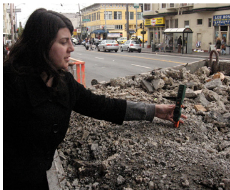
(a) A NoiseTube contributor measuring the level of environmental noise at a construction site using her mobile phone as a personal noise sensor instrument. The data is directly sent to the NoiseTube web application to update the exposure map of the city
