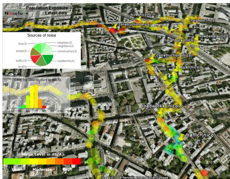
Figure 5.4: Visualisation using Google Earth representing the collective exposure to noise pollution generated by all the measurements and a tag cloud (shown as pie chart) with sources of noise
