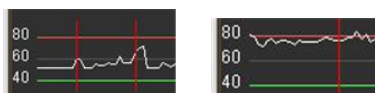
Figure 5.2: Screenshots of the noise exposure histogram in the phone UI, showing tagged events (red lines). The application can automatically tag different basic patterns of exposure such as sudden large variations in loudness or long lasting exposures to riskful loudness levels
